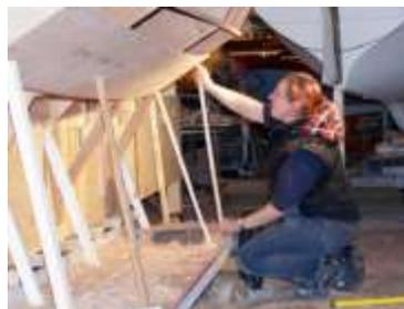
Below right Fran W is having a go at shaping the bevels on the Stem Post. In this one she is joining up the gaps left by Fred after he had cut to angles with his saw. Below left the stem has been generally bevelled and a dummy plank offered up to check how snug it fits. In the photo bottom right Ricky is busy locating the spiling plank in place so that we can take off the shape of the first plank. The spiling plank is a full length section of
