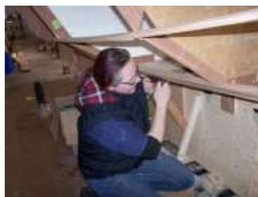
right Whaler John is checking the angle of the chine log making sure that he can nearly shave with the edge. Over left you can see a potential
