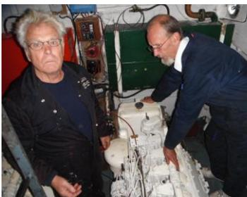
and didn’t need any assistance. In the photo bottom left under previous column Terry and Dave have replaced the water pump, Fred has tightened up all of the heat exchanger nuts in the hope that we had sorted out the issues. A brief run up the harbour proved the Starboard engine water pump but the port engine was still getting warm so Terry took out the thermostat so she would run cooler. Over left you can see the wake as Danny puts her through her paces so she was ready to take out the
