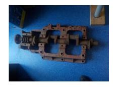
restoration of Falmouth. Work has also been started off site on her steam engine. Below left the photo shows part of her original engine. The plan is for the original engine to be rebuilt as a static display with a new replica steam engine being built for the operational aspects of the boat. The lower engine section shown here will be used as part of the detailed planning for the engine bed before being sent away to be incorporated in the static display engine.
