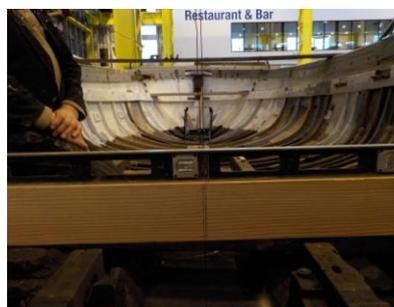
These are the ‘floor joists’ of the boating world. Over left John P is
